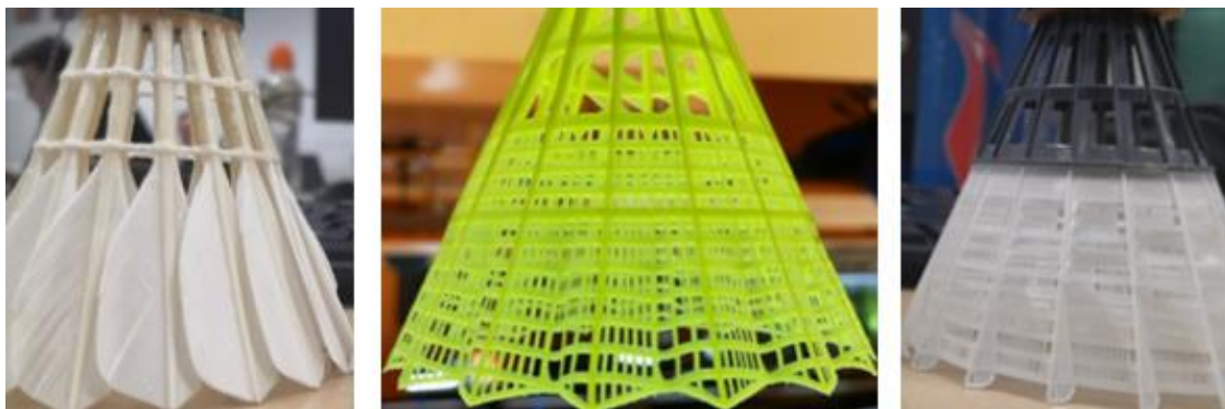
Figure 6. Comparison of skirt patterns of: a) Feather shuttlecock, b) Single-piece synthetic skirt and c) Two-piece synthetic skirt. Clear discrepancies can be observed not only between the feather and synthetic skirts, but also between the different synthetic shuttlecock brands.
